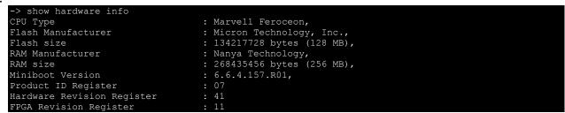
You can also view information for each switch in a stack (if applicable) using the show ni command as shown below.
